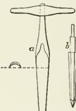
Broaches for Boring. Fig. a is an example of broaches or reamers for wood, and fig. b of those for metal.
